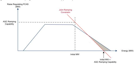
Similar diagrams can be drawn for the regulating lower service. For the regulating lower service, the joint ramping constraint would truncate the feasible solution area under the left-hand-side trapezium slope.
