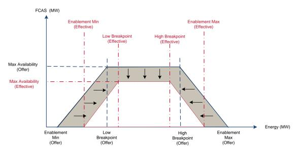
Table 1 summarises the range of intervals over which FCAS trapezium scaling applies in the Dispatch, Pre-dispatch and 5-minute Pre-dispatch processes.
