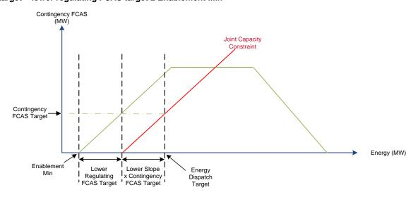
One consequence of these constraints is that the energy dispatch target is bound by the Enablement Min and the Enablement Max when a unit is enabled for contingency FCAS. This phenomenon is referred to as "trapped within the FCAS trapezium".
