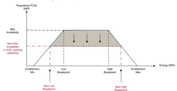
Figure 7: FCAS trapezium scaling by AGC ramp rates
