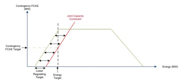
Joint capacity constraints are created for all units with an energy offer and which are enabled for a contingency service. One set of constraints is created for each contingency service (fast raise, slow raise, delayed raise, fast lower, slow lower, or delayed lower) for which the unit is enabled. The joint capacity constraint equations for each type of contingency FCAS are:
