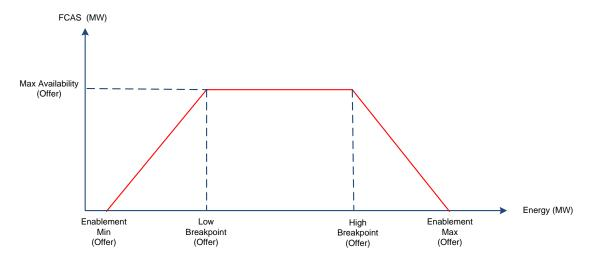
The technical limits submitted as part of an FCAS offer must be within the bounds of the technical envelope specified during registration of that provider for that FCAS.
