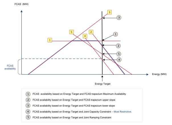
FCAS availability for each FCAS can be calculated using the formula below. The formula incorporates the FCAS trapezium scaling. For each limit equation, the corresponding constraint type is marked from to 5.
