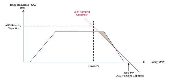
Figure 12: Joint ramping constraint - shallow upper slope
