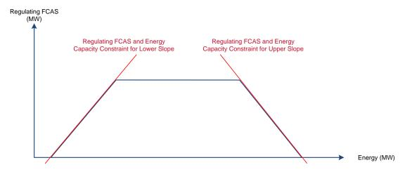
One consequence of these constraints is that the energy dispatch target is bound by the Enablement Min and the Enablement Max when a unit is enabled for regulating FCAS. As with contingency FCAS, this phenomenon is referred to as "trapped within the FCAS trapezium".
